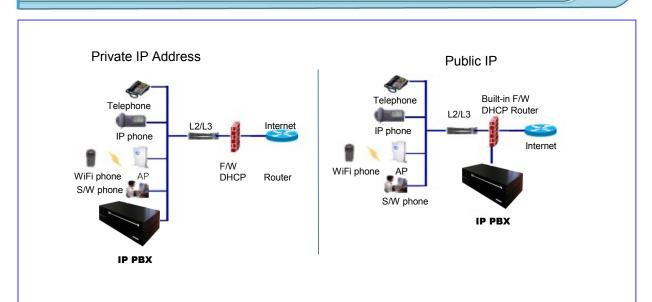
• Can be configured for both private and public IP network configuration. Automatically supports and configures NAT, the IP-PBX comes with built-in firewall, DHCP, VLAN and NTP modules.
